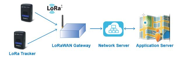
Before starting communication LoRaWAN Gateway and LT-100 LoRa trackers, please refer to the LoRaWAN gateway's user manual to set the LoRa settings described on "4. LoRa settings" by GlobalSat-LT-100 Config Tool.
