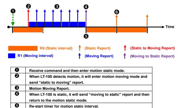
You could define the content of report and the report interval of motion mode. You could set LT-100 to be motion mode by setting parameter O4=4 via configuration tool.
